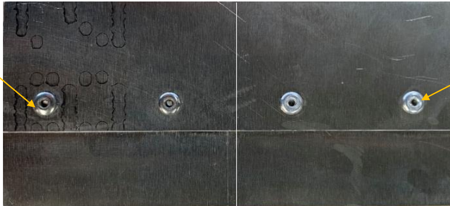
Figure 4 – Identification of stainless steel and aluminium rivets
