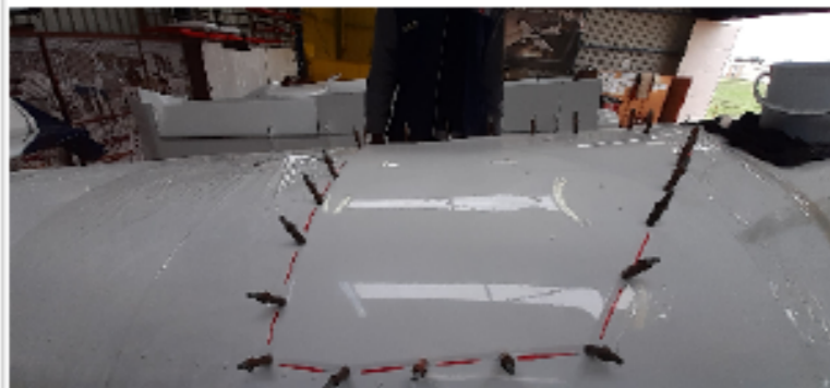
Example of tracing the Blowout skin to the Rear Fuselage
