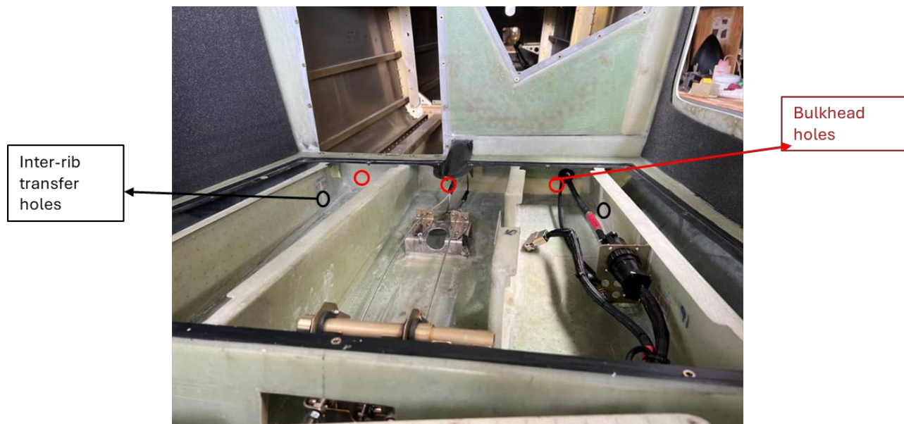
Figure 17: Imagery illustration (Bulkhead and inter-rib transfer holes for both configurations)
