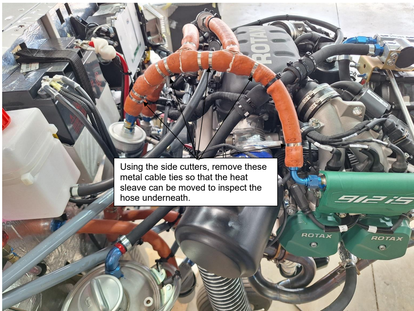
Figure 6: Example of cable ties to be removed.
