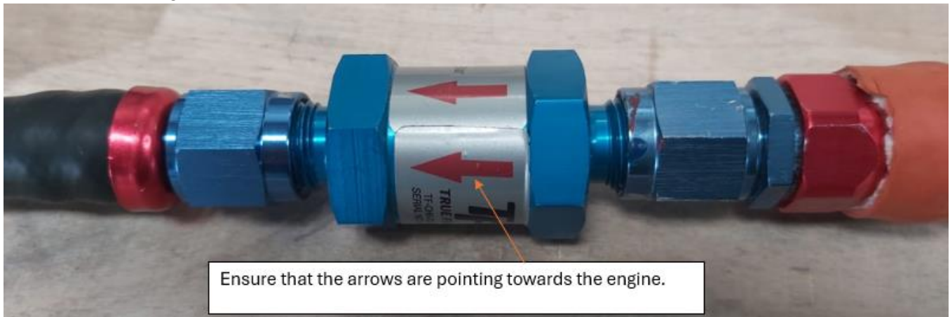
| Figure 5: Ensure that the arrows are pointing towards the engine.
