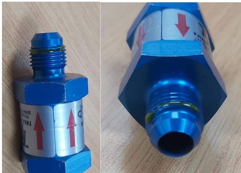
Figure 4: Check Valve with a thin layer of Loctite 577 applied on one thread and covering only half a turn.
