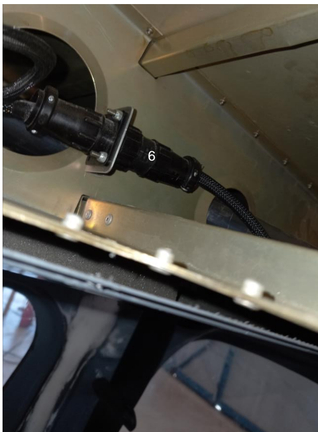
Figure 22: Flap actuator motor removal.
