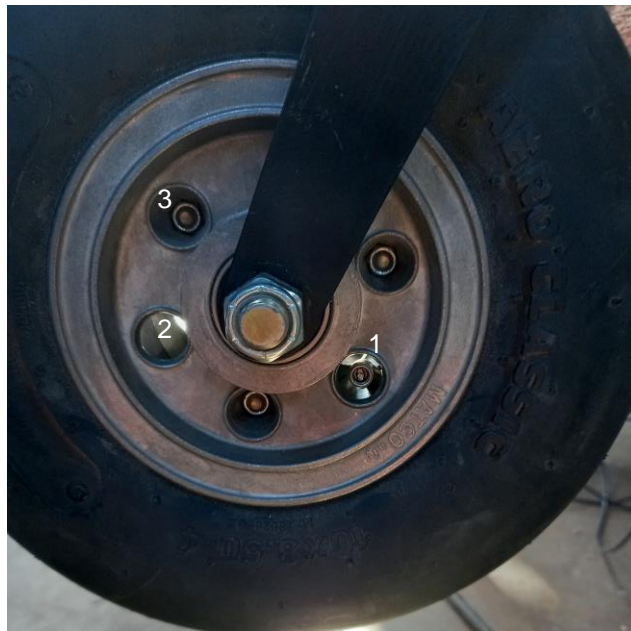
Figure 46: Tail wheel bolt placement
