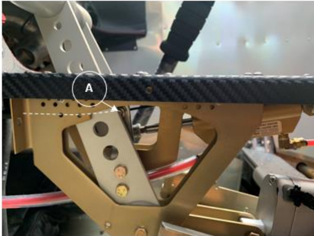
Figure 53: Inspect inner cable for kinking
