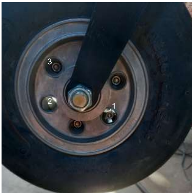
Figure 46: Tail wheel bolt placement
