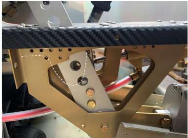
Figure 53: Inspect inner cable for kinking
