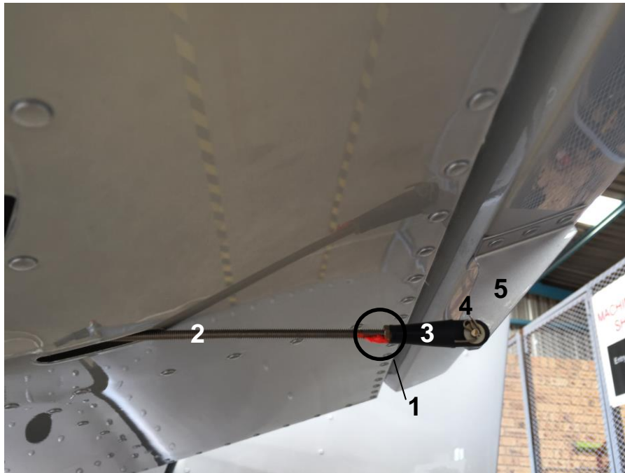
Figure 31: Elevator control horn (5)
