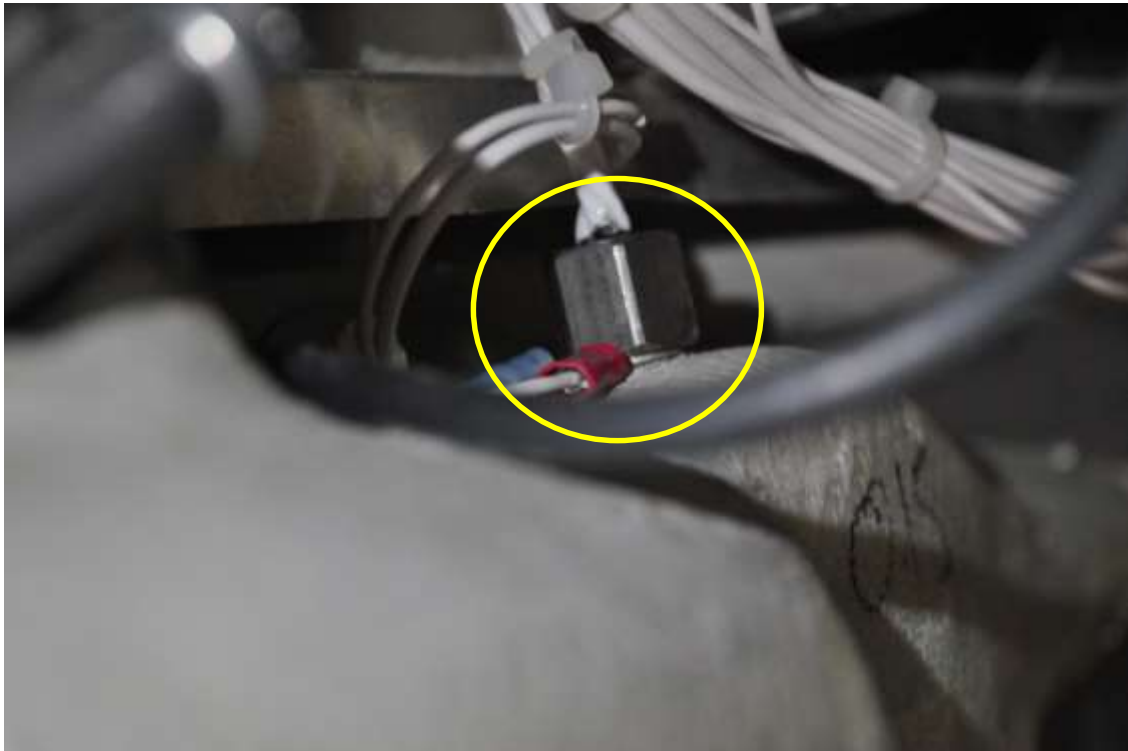
Figure 1: Grounding wire attached to the OAT probe
