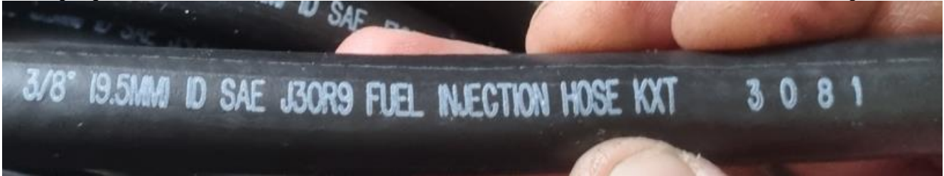
Figure 1: Sub-standard fuel hose - stamped lettering
