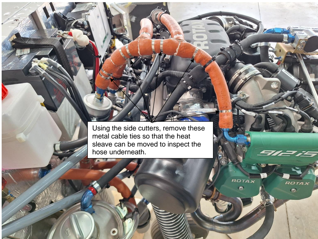
Figure 5: Example of cable ties to be removed.
