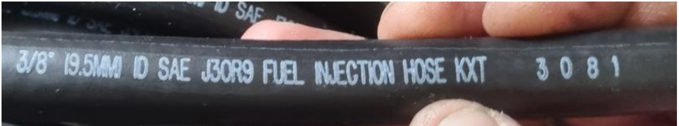
Figure 1: Sub-standard fuel hose - stamped lettering
