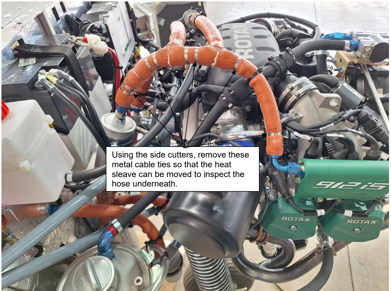
Figure 6: Example of cable ties to be removed.
