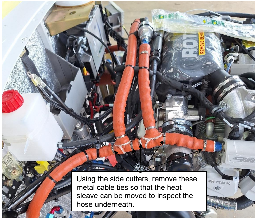
Figure 10: Example of cable ties to be removed.
