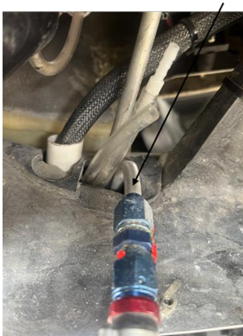
Front pillar close-up view showing typical sealing point
