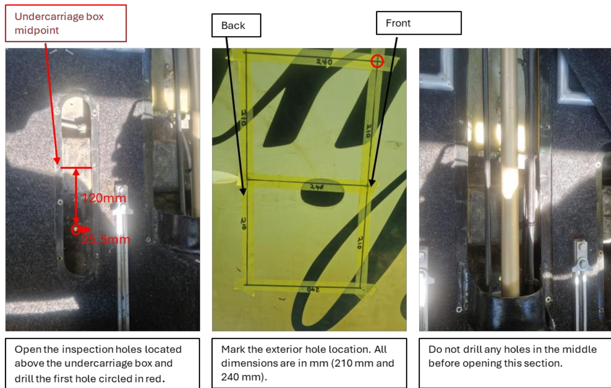
Figure 16: Imagery illustration (Tricycle belly drain holes)
