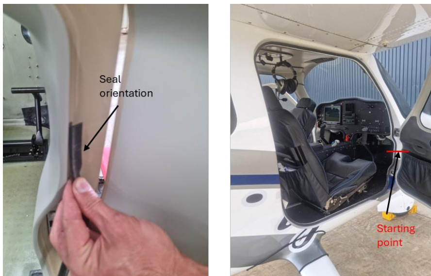
Figure 14: Door seal installation
