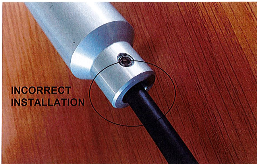
Figure 1 shows no steel end piece protruding and indicates an incorrect installation.
