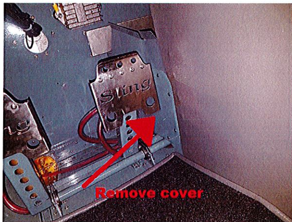
Figure 1 – Illustrates the covers to be removed
