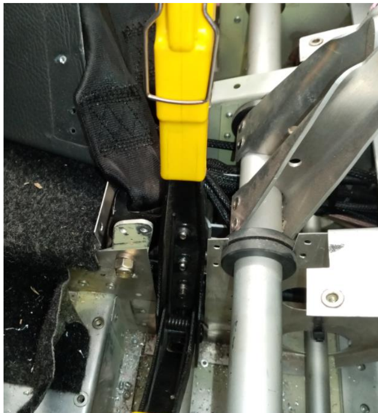
Figure 7 – Installation of stainless steel rivets
