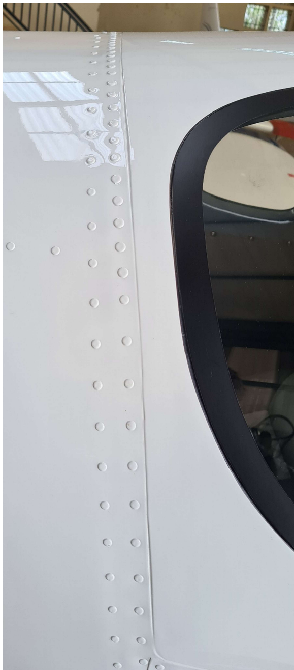
FIGURE 2 | CORRECT SPACING
