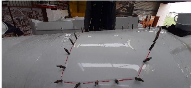
Figure 4: Tracing of the blowout skin on the rear fuselage
