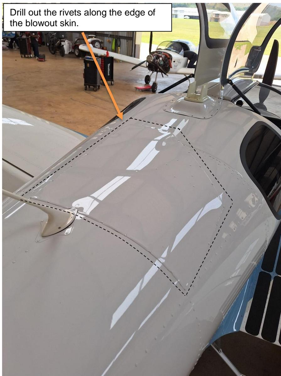
Figure 1: Blowout skin rivets to remove.
