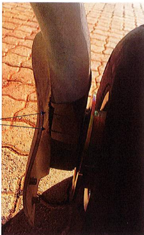
Figure 3 – Installed heat shield
