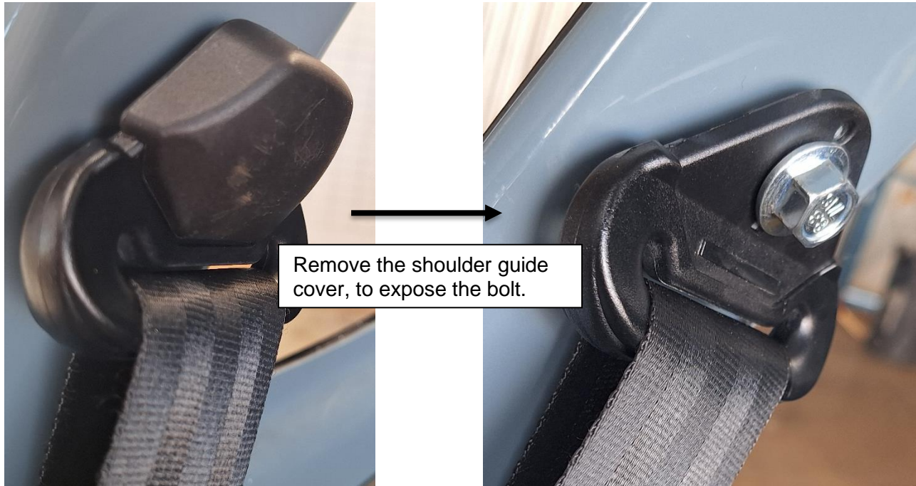
Figure 3: removal of the shoulder guide cover
