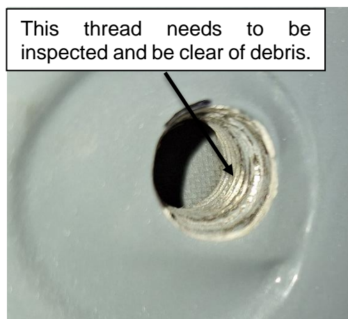
Figure 14: Threads to be inspected and tapped.
