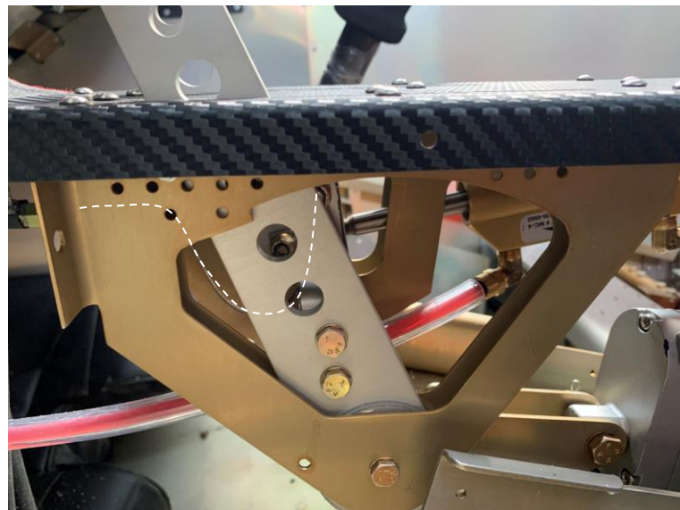
Figure 2: Inspect inner cable for kinking
