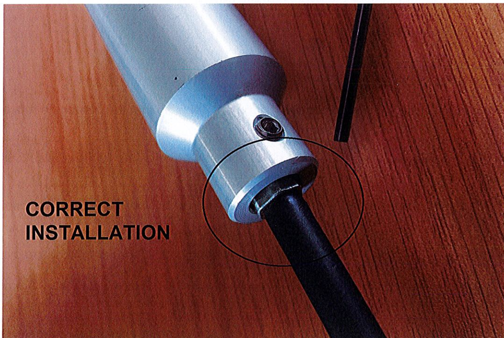
Figure 2 shows the steel end piece protruding out of the rocket base and indicates a correct installation.
