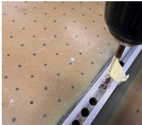
Figure 10: Additional anchor point hole drilling.
