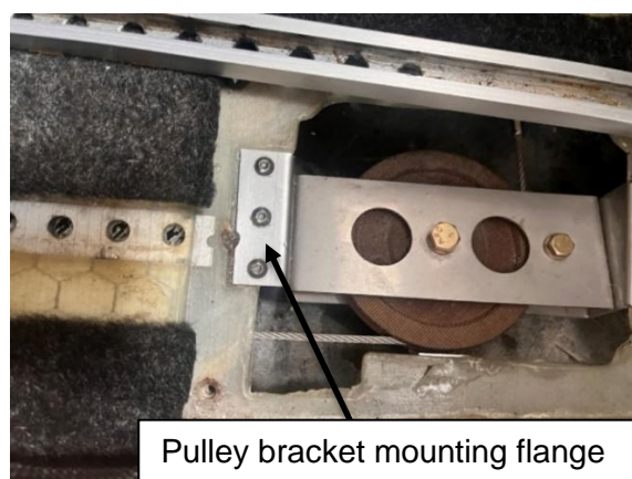
Figure 8: Photograph with inspection hatch removed.
