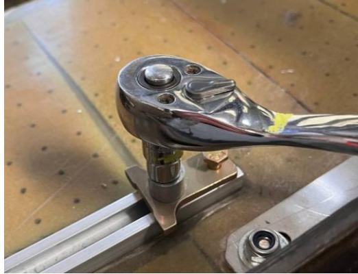
Figure 3: Rail bolt removal.
