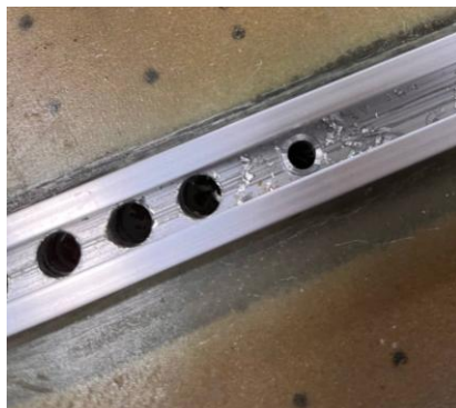
Figure 11: Additional anchor point hole countersinking.
