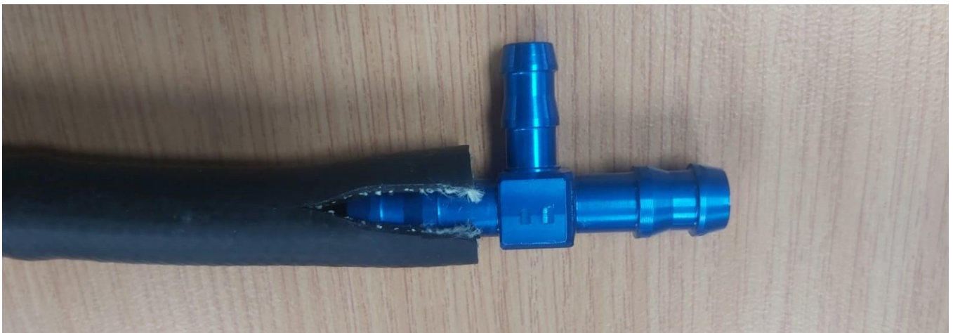
Figure 4: Illustration of the lengthwise cut through the hose.
