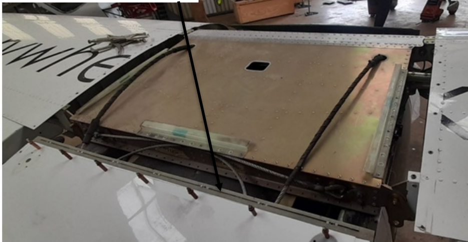
Figure 14: The joggle should be 30mm wide for the removable roof to fit properly.
