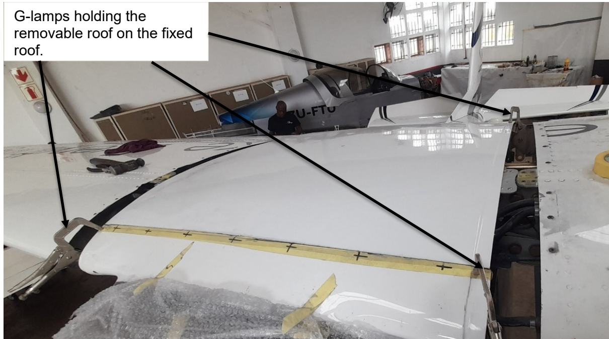
Figure 2: G-lamps holding the removable roof on the fixed roof to measure cut lines.
