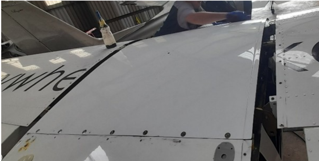
Figure 31: Removable roof installed on the fuselage.
