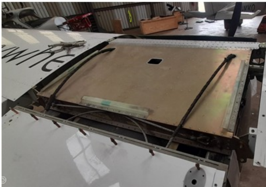
Figure 5: The fixed roof removed from the fuselage
