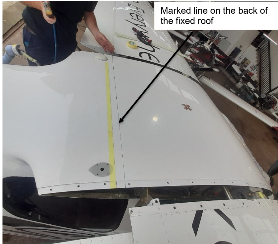
Figure 3: Marked line on the back of the fixed roof.
