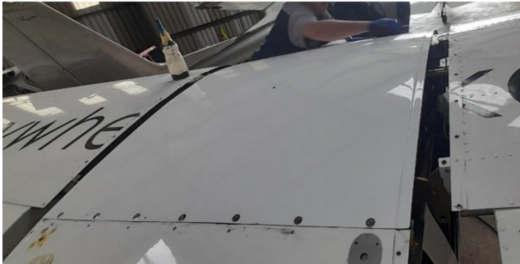
Figure 28: Installed removable roof on the fuselage.
