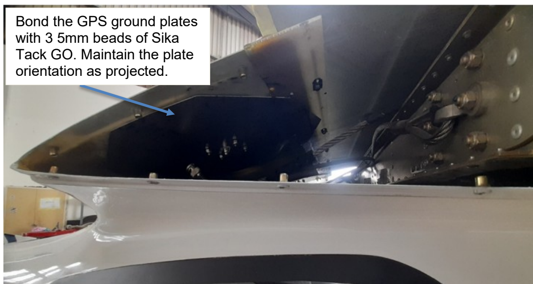
Figure 26: GPS Plate bonded on the rear roof panel.
