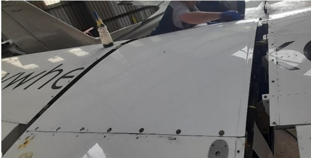
Figure 21: Installed removable roof on the fuselage.
