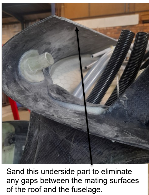
Figure 9: Front section where the removable roof intercept with the fuselage.
