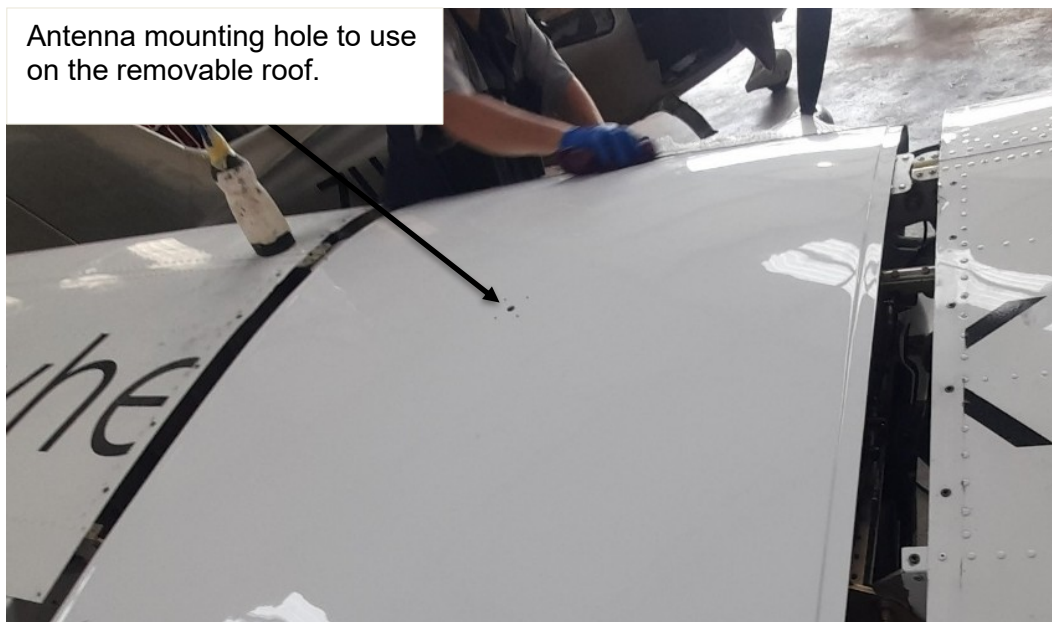
Figure 6: Antenna mounting hole to use on the removable roof.
