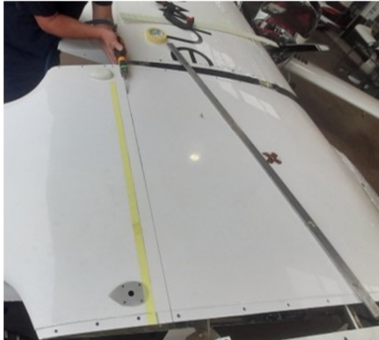
Figure 4: Cutting of the fixed roof on the line marked.
