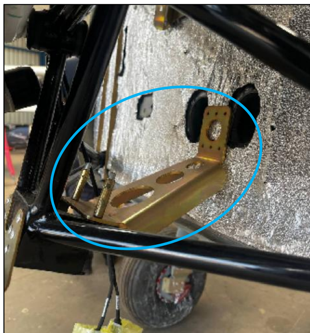
Figure 5. Old/Current Bellcrank Support Bracket to be Removed.
