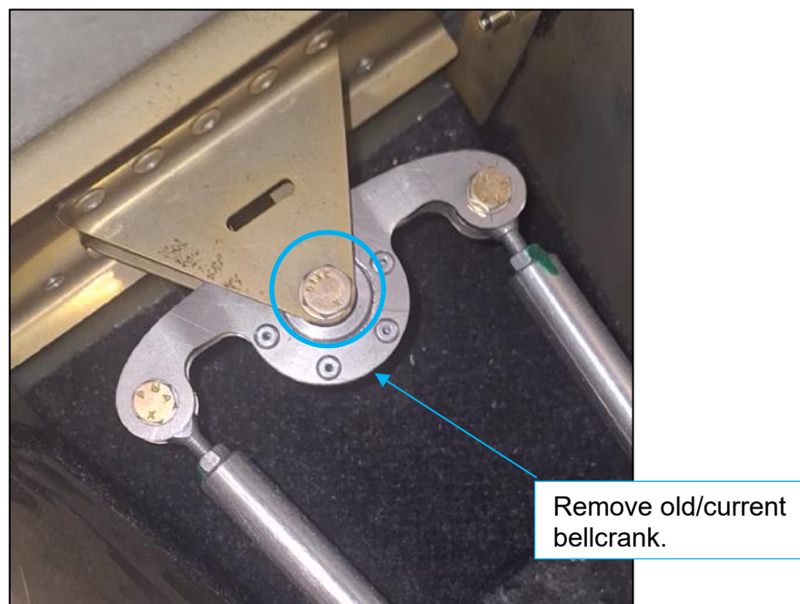
Figure 3. Removal of Old/Current Bellcrank.
