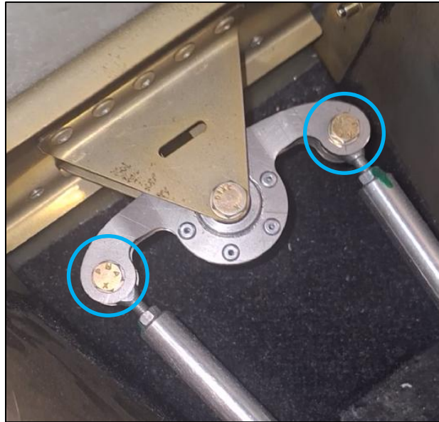
Figure 2. Bolts to Remove for Detachment of Pedal Pushrod Assemblies.
