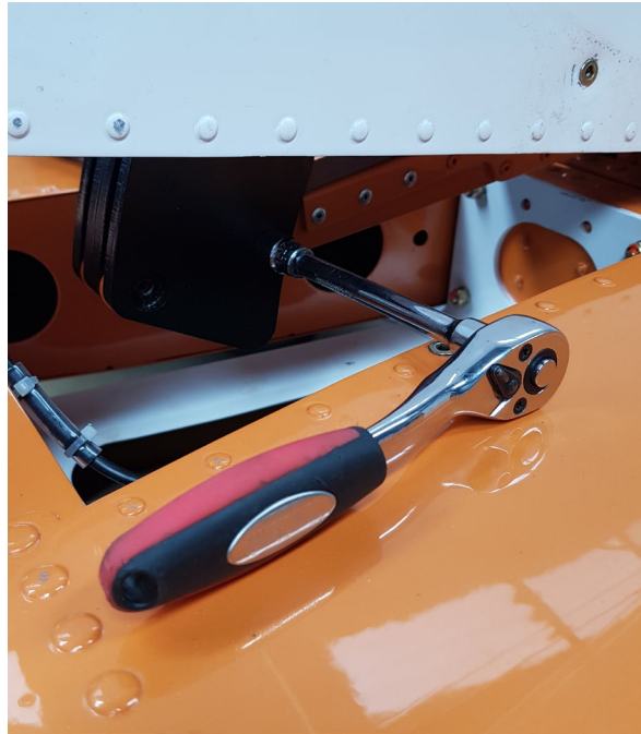
Figure 2 Removal of the balance weight bolts
