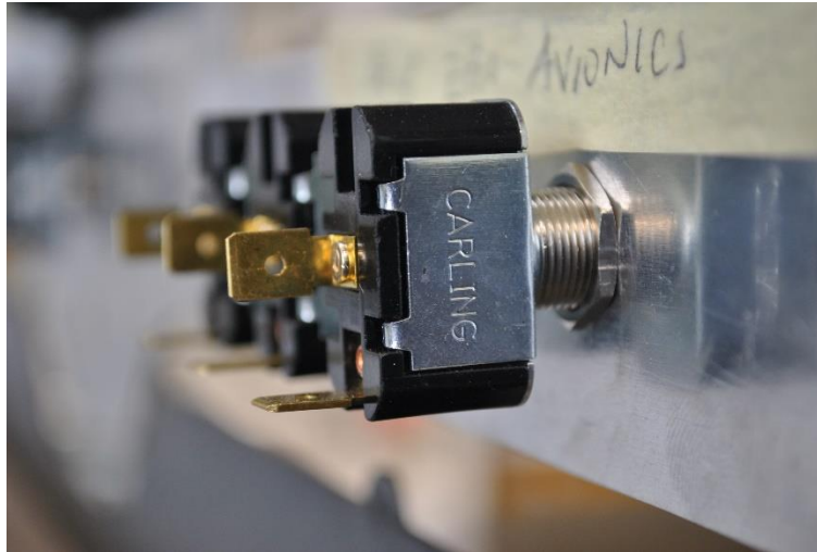
Figure 1: Incorrect master switch
