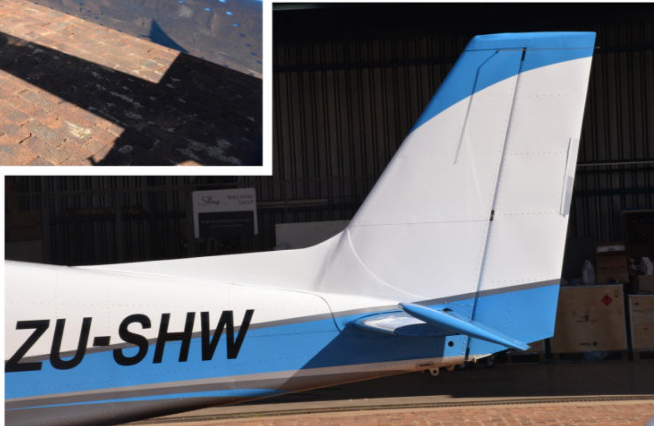
RIGHT: Designers found that at higher angles of attack, directional control was compromised by blanking of the tail by the fuselage. A taller vertical and rudder solved the issue and still looks very Sling-like.
