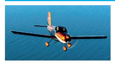
ntroduced in mid-2017, the RV-12iS was a revised version of the original RV-12. The -12iS was designed specifically to meet the US Light Sport Aircraft regulations, and for a 100hp sport aircraft, delivers some great numbers. With its 336kg empty weight, you can carry two 90kg crew, full fuel (75 litres), and still bring some baggage and not exceed max gross weight.
