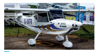
The Mission M108 is available as a complete kit. the basic price for which starts at €61,500 ex.VAT. For that you get a complete package including airframe, systems, powerplant and propeller. All fuselage welding is done and powder coated, and the wing structure is partially assembled. Once the airframe is complete, it's time to use your fabric-covering skills.
