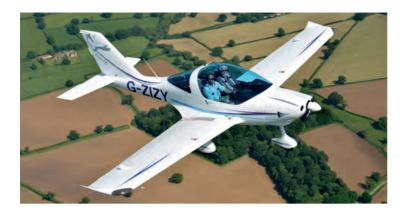
ne of only two composite kits that features in our list, the Sting S4's carbon airframe comes pre-finished in white, that might seem like a small point, will save a builder the additional cost of painting when the aircraft is complete. The low-wing, side-by-side two-seater can be powered by the Rotax 912ULS or 912iS. The tapered wings are detachable, glider-style.
