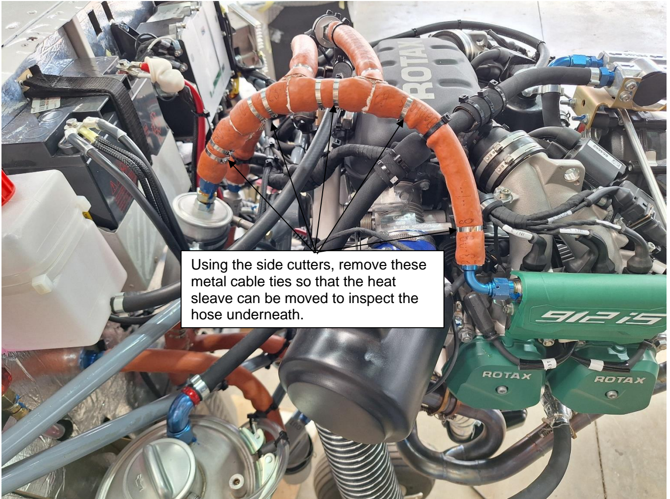
Figure 6: Example of cable ties to be removed.
