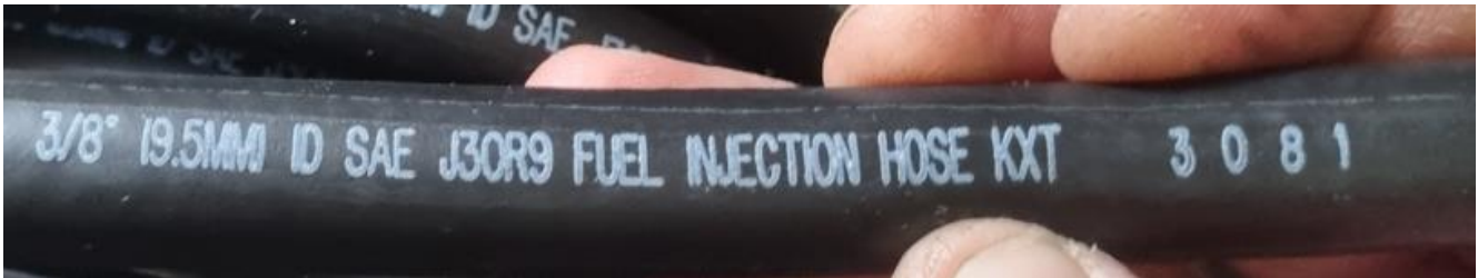
Figure 1: Sub-standard fuel hose - stamped lettering
